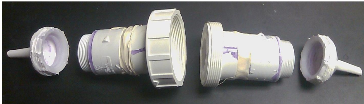
Figure 4.2. Image of sampler V2, dismantled to illustrate different components. Inlet is on the left side. Woven wire mesh is placed in center section before fastening left and right sections together.
